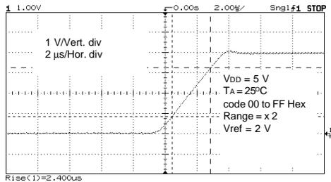
Rise time = 3.75  $\mu\text{s}$ , Positive slew rate = 0.54  $\mu\text{s}$
