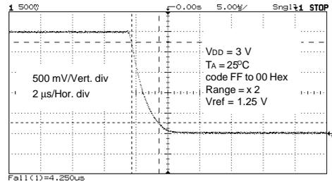
Fall time = 4.85  $\mu\text{s}$ , Negative slew rate = 0.41  $\mu\text{s}$
