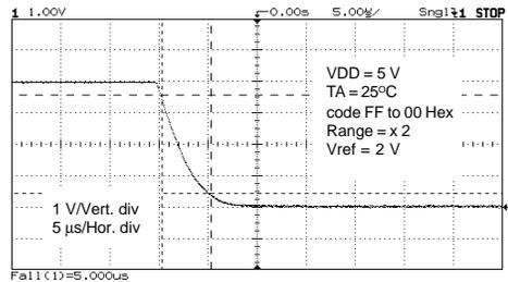
Fall time = 5.9  $\mu\text{s}$ , Negative slew rate = 0.54  $\mu\text{s}$
