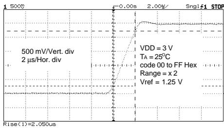
Rise time = 2.5  $\mu\text{s}$ , Positive slew rate = 0.80  $\mu\text{s}$
