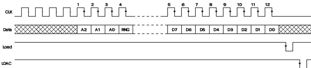
Figure 4. LDAC controlled update using 8-bit serial word.
