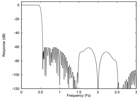
Figure 7 DAC Digital Filter Frequency Response
