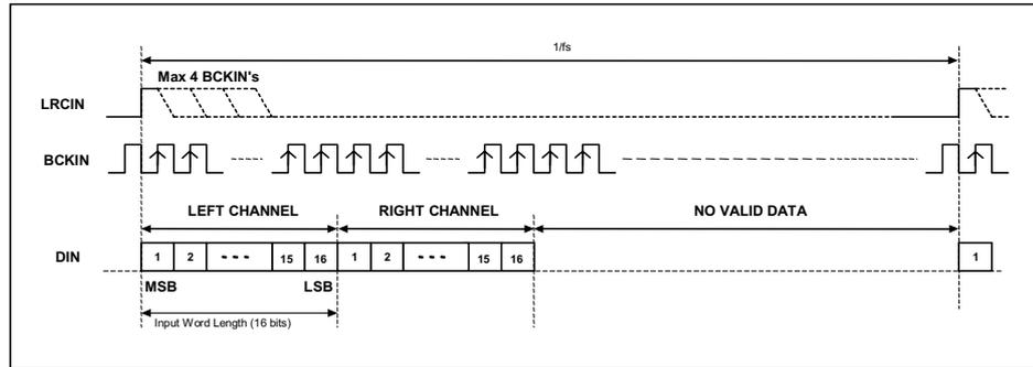
Figure 5 DSP 'Late' Mode Timing
