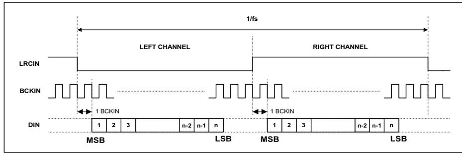
Figure 3 I²S Mode Timing Diagram
