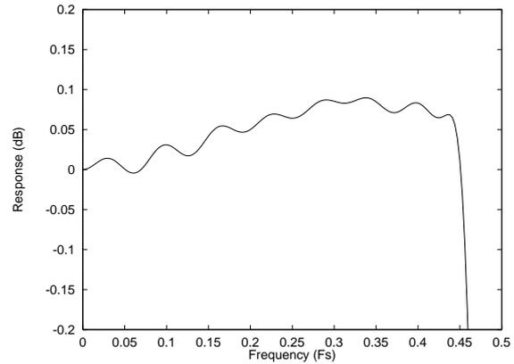
Figure 8 DAC Digital Filter Ripple
