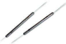
OPLINK 1550/1625nm WDMs are manufactured by using the proven fused biconical taper technology and OPLINK stringent quality procedures. With low insertion loss and flat passband, this device is ideal for combining or separting light signals in the 1550 and 1625 nm bands.
