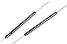
OPLINK 980/1550nm WDMs are manufactured by using the proven fused biconical taper technology and OPLINK stringent quality procedures. With low insertion loss and flat passband, this device is ideal for combining pump (980 nm) and signal light at 1550 nm in optical fiber amplifiers.
