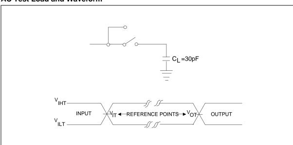
AC test inputs are driven at VIHT (0.9 VDD) for a logic "1" and VILT (0.1 VDD) for a logic "0". Measurement reference points for inputs and outputs are at VIT (0.5 VDD) and VOT (0.5 VDD) Input rise and fall times (10%  $\leftrightarrow$  90%) are <5 nS.
