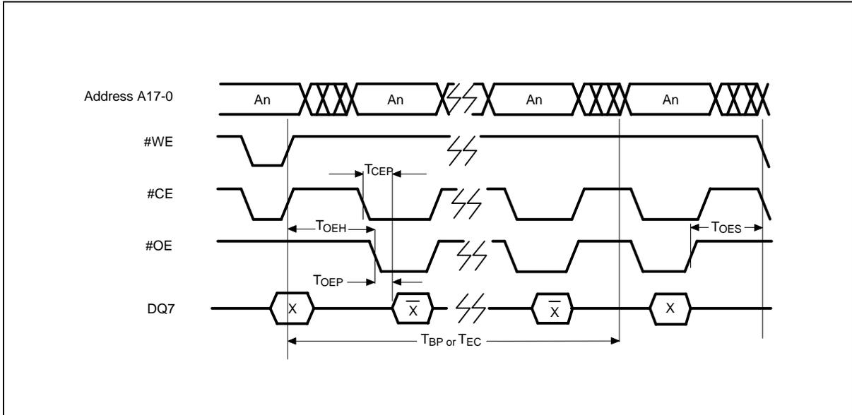
**Toggle Bit Timing Diagram**
