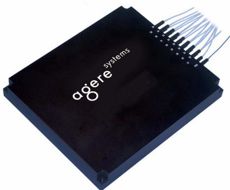
The W7200-type 200 GHz thin-film multiplexers (MUX) and demultiplexers (deMUX) are characterized by high-adjacent and nonadjacent channel isolation, excellent directivity, and very low optical loss values.
