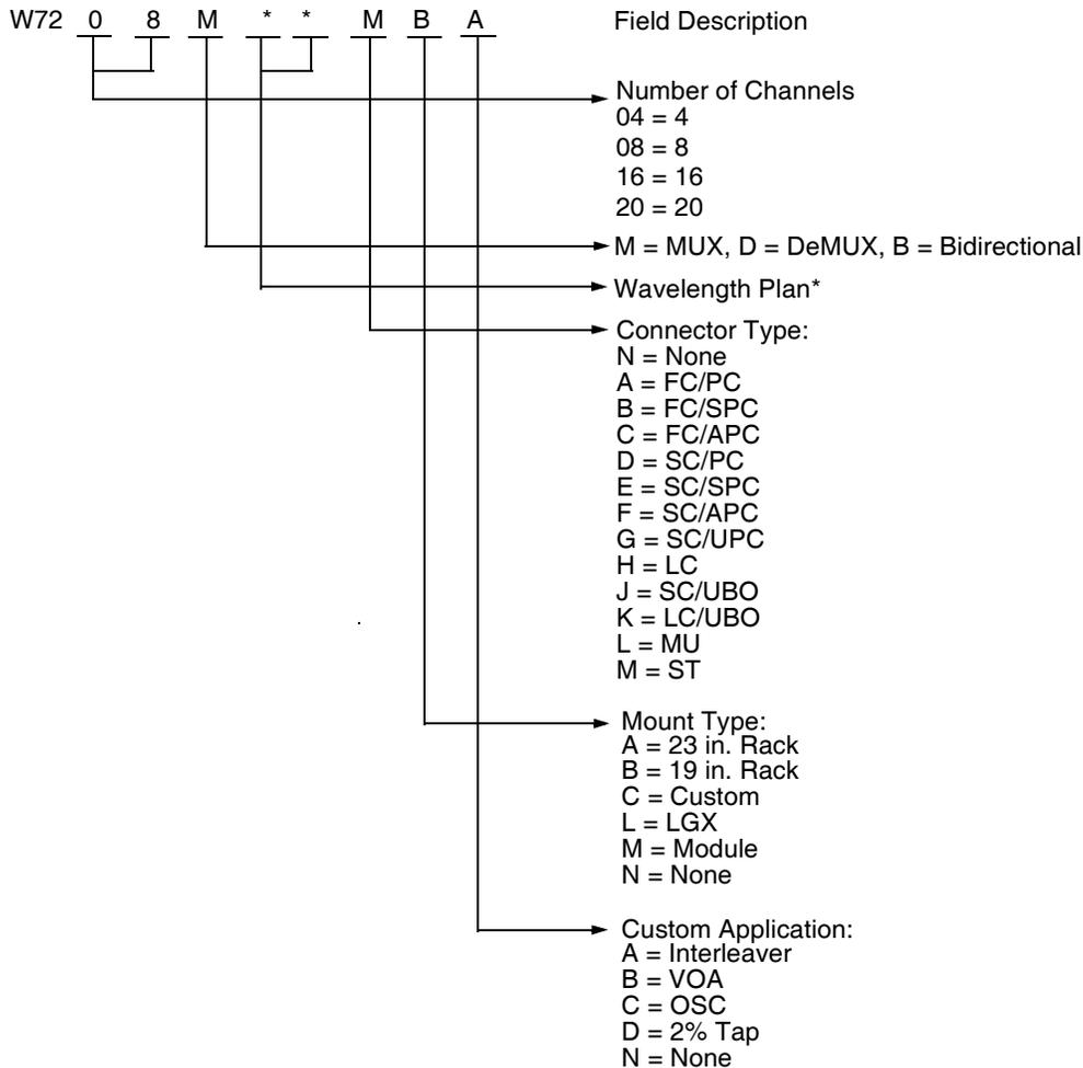
Example: W7208M\*\*MBA represents an eight-channel multiplexer with custom wavelength plan, ST connector, and 19 in. mounting rack; intended for interleaver applications.
