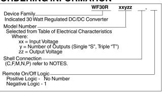
NOTES: A "C" designator indicates the aluminum shell is connected internally to the common output return pin.
