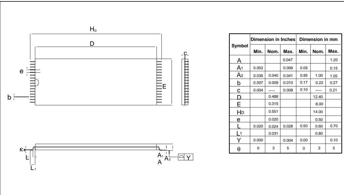
The diagram illustrates the 32-Lead Small Type One TSOP package. The top view shows the overall package dimensions: D (width), H<sub>D</sub> (height), b (lead pitch), e (lead height), and C (lead spacing). The lead detail view shows the lead profile with dimensions A, A<sub>1</sub>, A<sub>2</sub>, L, L<sub>1</sub>, and Y. Pin 1 is indicated at the bottom right.
