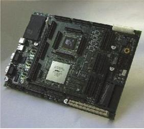
SIDSA has recently launched the HSDT200 ARM Emulation Board for embedded ASIC prototyping and software integration.
