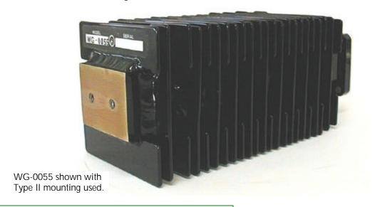
Microlab/FXR WG series dummy loads are optimized versions of the DA loads per MIL-D-3954A or their commercial equivalents. Superior performance is achieved by slight changes in physical dimensions, more efficient fin cooling and increased waveguide pressure. Also, additional mounting in the form of tapped holes with stainless steel inserts are provided at the rear of the loads.
