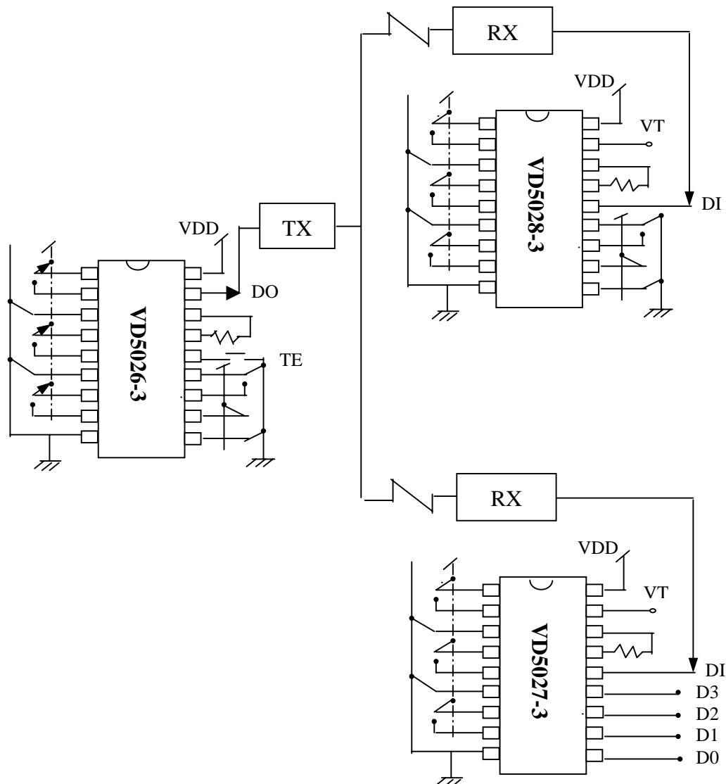
The IC substrate should be connected to V<sub>DD</sub>. 芯片襯底請接V<sub>DD</sub>。
