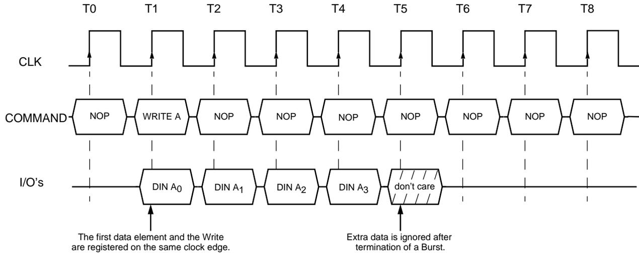
6.1 Write Interrupted by a Write
