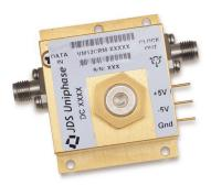
This product is used to generate a high-level synchronous clock signal from 12 Gb/s return-to-zero (RZ) or NRZ data. This module includes a temperature stable high "Q" filter (800 to 1000) for excellent jitter transfer characteristic, which unlike phase-locked-loop designs cannot "loose lock."
