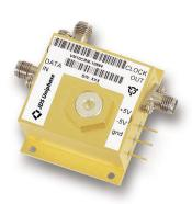
This product is used to generate a high-level synchronous clock signal from 10 Gb/s NRZ data. This module includes a temperature-stable high "Q" filter (800 to 1000) for excellent jitter transfer characteristic, which unlike phase-locked-loop designs cannot "loose lock."
