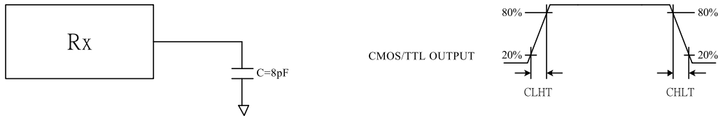
Figure 2. Receiver CMOS/TTL Output Load and Transition Times
