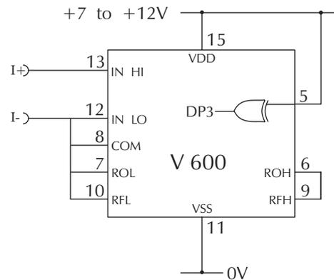
Measuring a current referenced to a floating supply, i.e. the current being measured and the meter's power supply are isolated from each other.
