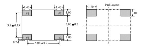
Note: Depending upon electrical options, different program layout may be used. However, both are compliant to the connection and pad layout of the above.
