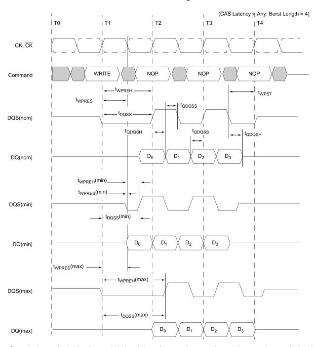
Once the burst of write data is concluded and given that no subsequent burst write operations are initiated, the data strobe signal (DQS) transitions from a logic low level back to Hi-Z. This is referred to as the data strobe "write postamble". This transition happens nominally one-half clock period after the last data of the burst cycle is latched into the device.
