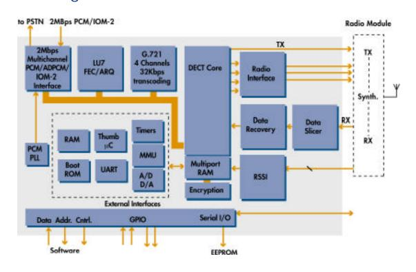
Processor. The core supports fully programmable B-field sizes, permitting half-, full- and double-slot operation, as well as allowing mixed slot sizes within a single TDMA frame. This flexibility allows manufacturers to implement powerful data features, including 64 kbps data support. In the Vega VMax device this 64 kbps support is enhanced by the inclusion of a Reed-Solomon coder supporting the ETSIdefined LU7 64 kbps data profile, thus allowing ISDN signals to be sent seamlessly over DECT.
