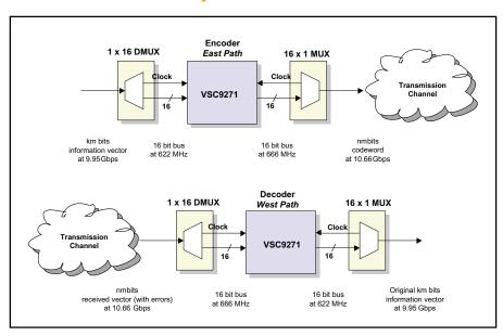
The bi-directional architecture of the VSC9271 allows for complete East/West monitoring on ring traffic, or dual channel operation. The count of corrected ones and zeros provided by the VSC9271's FEC can be used as a protocol independent channel monitor, allowing for completely transparent monitoring of any incoming signal independent of the rate or protocol.
