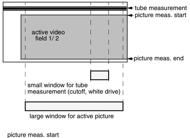
**Fig. 2–21:** Windows for tube and picture measurements
