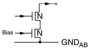
Fig. 6–16: Output pins ROUT, GOUT, BOUT, SVMOUT
