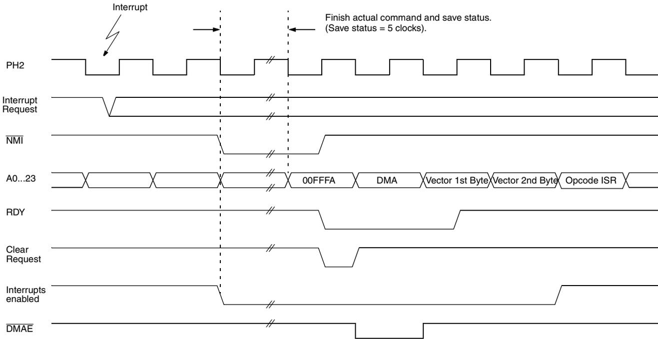
**Fig. 5–15:** Interrupt timing diagram
