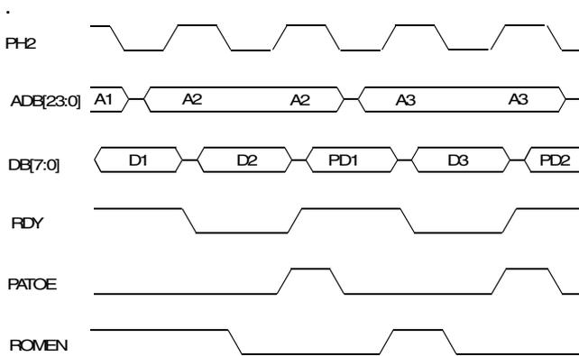
Fig. 5–17: Patch timing
