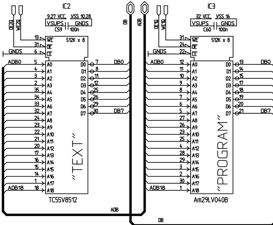
Fig. 7-3: VCT 38xxA application circuit, part 3/3
