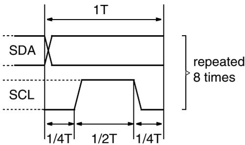
Fig. 5–20: Single bit on I<sup>2</sup>C bus
