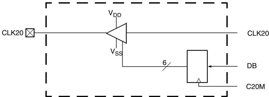
**Fig. 5-8:** CLK20 Port Circuit
