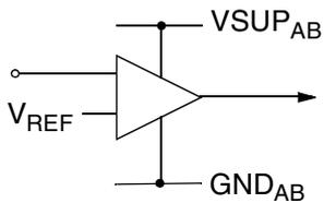
Fig. 6–19: Input pin FBLIN
