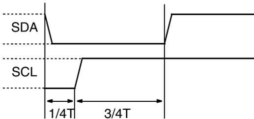
Fig. 5–21: Stop condition I<sup>2</sup>C bus
