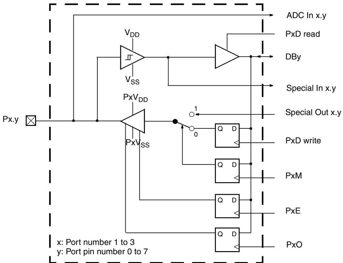
**Fig. 5–5:** Universal port circuit
