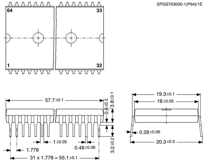
**Fig. 6-1: 64-Pin Plastic Shrink Dual-Inline Package (PSDIP64)**
