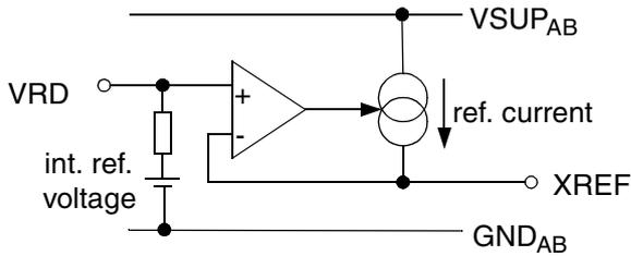
**Fig. 6-25:** Supply pins XREF, VRD
