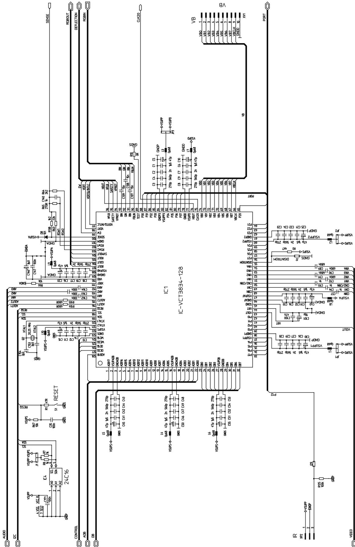
Fig. 7-1: VCT 38xxA application circuit, part 1/3
