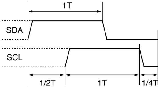
Fig. 5–19: Start condition I<sup>2</sup>C bus
