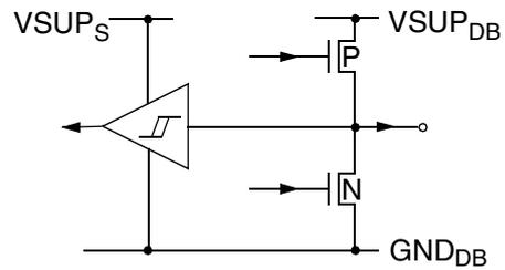
**Fig. 6-31:** Input/Output pins DB0-DB7
