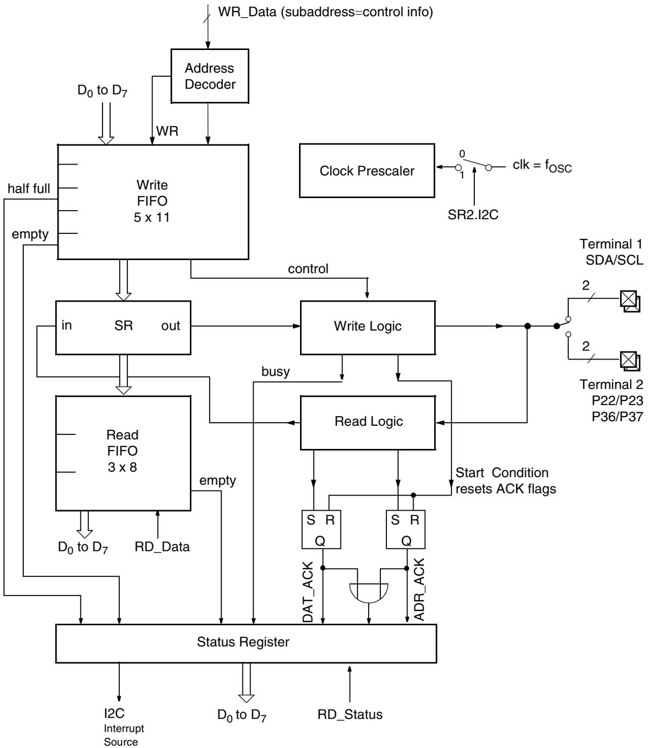
Fig. 5-18: Block diagram of I<sup>2</sup>C bus master interface
