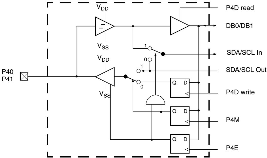
**Fig. 5-6:** I<sup>2</sup>C port circuit
