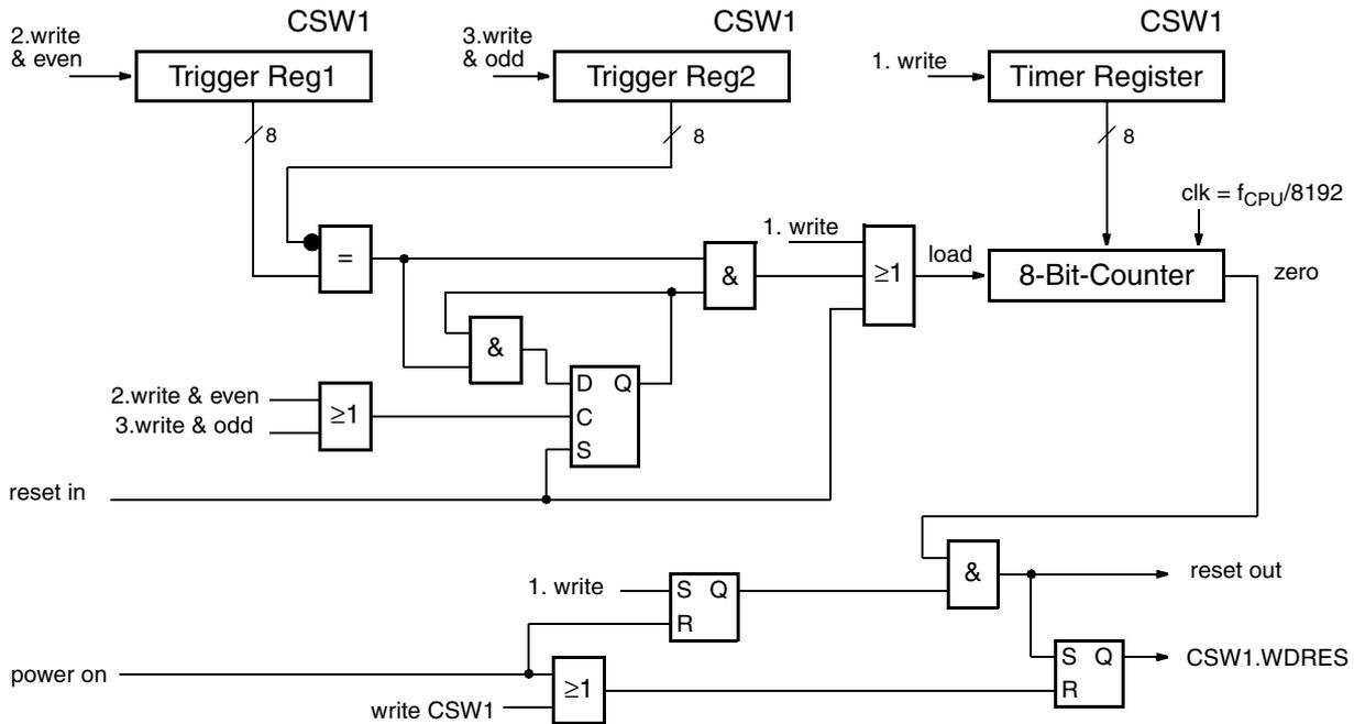
Fig. 5–4: Block diagram of watchdog
