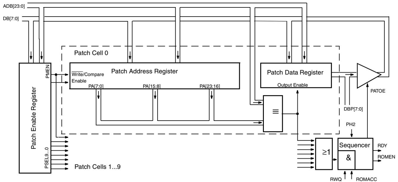
Fig. 5–16: Block diagram of patch module
