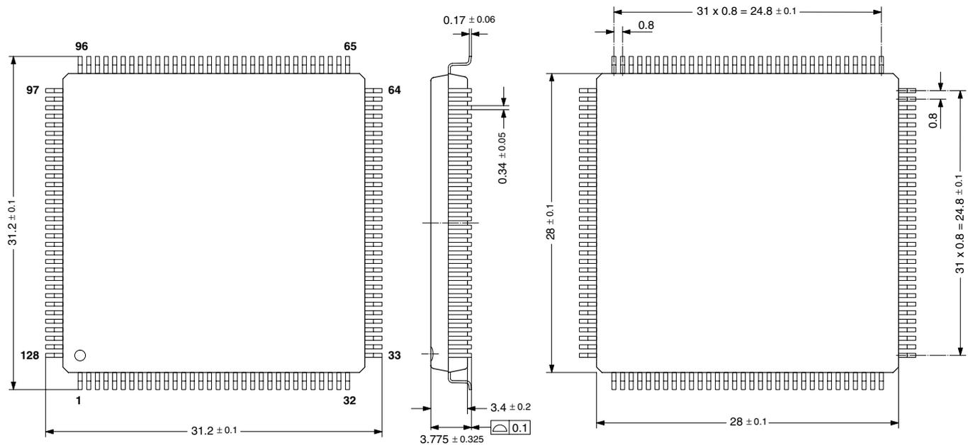
**Fig. 6-2: 128-Pin Plastic Metric Quad Flat Package (PMQFP128)**
