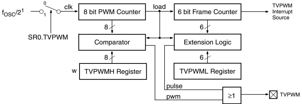
**Fig. 5–2:** Block Diagram of 14bit Tuning Voltage PWM
