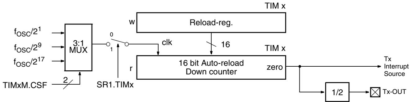
**Fig. 5–22:** Block diagram of timer T0 and T1
