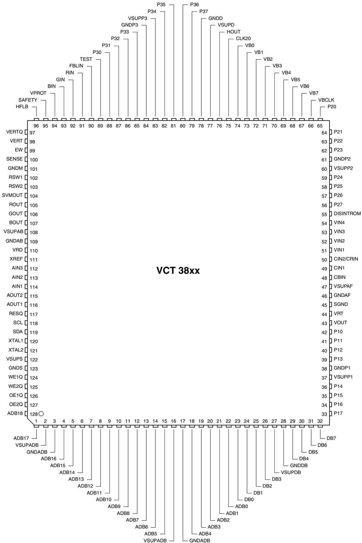
**Fig. 6-5:** 128-pin PMQFP package
