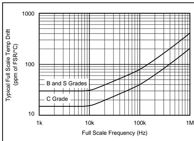
Figure 3. Full Scale Drift vs Full Scale Frequency.
