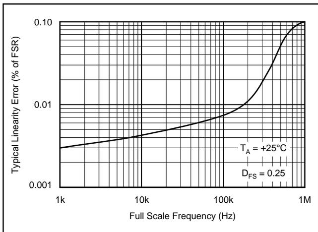
Figure 1. Linearity Error vs Full Scale Frequency.
