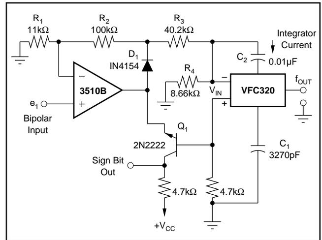
FIGURE 14. Absolute value circuit with the VFC320. Op amp,  $D_1$  and  $Q_1$  (its base-emitter junction functioning as a diode) provide full-wave rectification of bipolar input voltages. VFC output frequency is proportional to  $|e_1|$ . The sign bit output provides indication of the input polarity.
