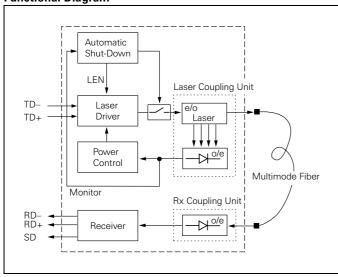
The receiver component converts the optical serial data into PECL compatible electrical data (RD and RDnot). The Signal Detect (SD, active high) shows whether an optical signal is present.
