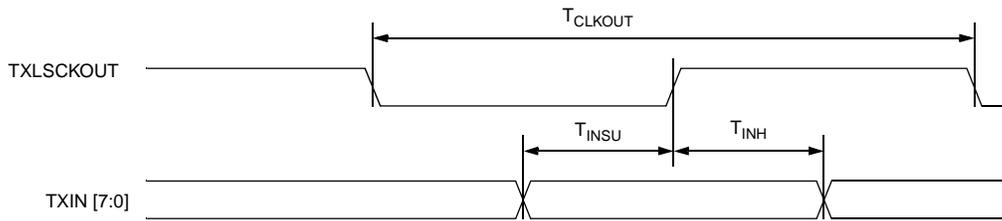
**Table 6: Transmit Data Input Timing Table (STS-12 Operation)**
