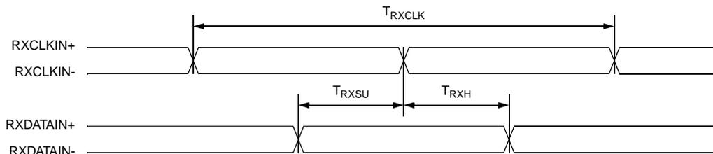
**Table 4: Receive High Speed Data Input Timing Table (STS-12 Operation)**
