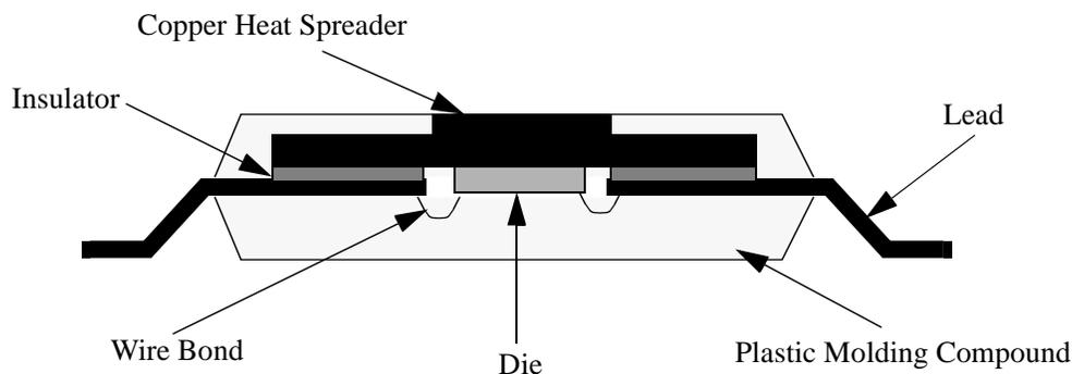
The thermal resistance for the VSC8116 package is improved through low thermal resistance paths from the die to the exposed surface of the heat spreader and from the die to the lead frame through the heat spreader overlap of the lead frame.
