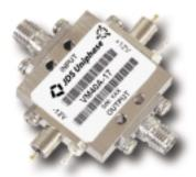
The JDS Uniphase VM40A small signal amplifier is a gain block designed to boost the signal level generated at the optical to electrical receiver stage (PIN/APD). It is capable of reproducing a sinusoidal EYE pattern signal running at OC768 data rates, with an output level up to 2 Volts peak-to-peak maximum.
