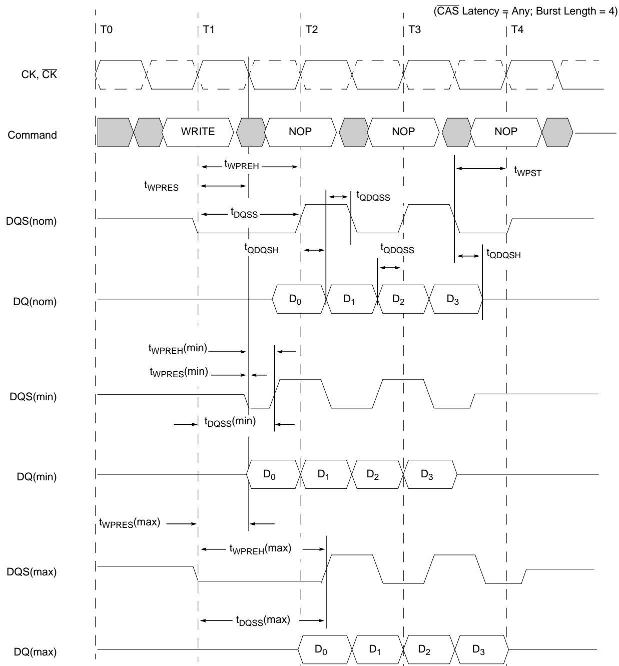
Once the burst of write data is concluded and given that no subsequent burst write operations are initiated, the data strobe signal (DQS) transitions from a logic low level back to Hi-Z. This is referred to as the data strobe "write postamble". This transition happens nominally one-half clock period after the last data of the burst cycle is latched into the device.
