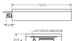
Electrical connector is 12-pin right-angle header (Molex part number 22-12-2124). Mate with Molex part number 22-01-3127 or equivalent.
