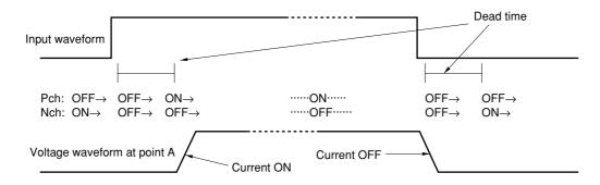
Output A goes into a high-impedance state and is in an undefined status during the dead time period. Because output B is pulled down by the load, a low level is output to A.
