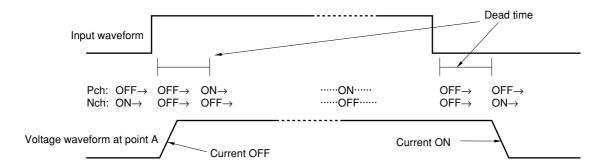
Output A goes into a high-impedance state and is in an undefined status during the dead time period. Because output B is pulled up by the load, a high level is output to A.
