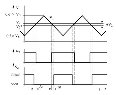
Figure 4. Signal characteristics of pulse width control with time window generation
