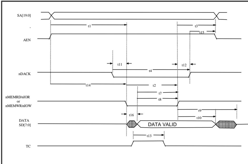
FIGURE 13 - DMA TIMING (SINGLE TRANSFER MODE)
