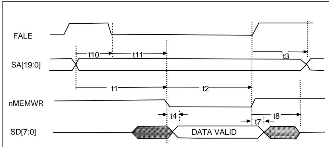
**FIGURE 17 - 8051 FLASH MEMORY WRITE TIMING**
