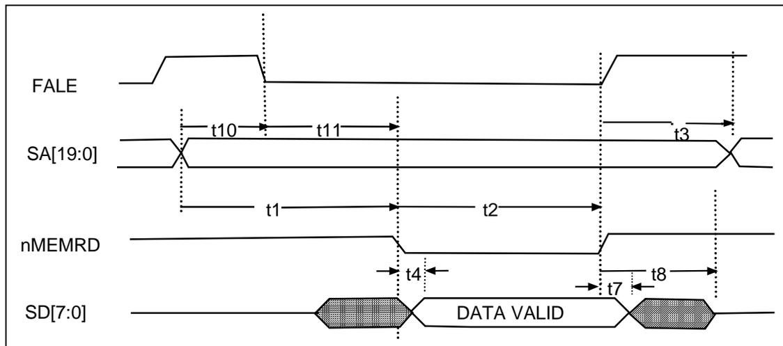
FIGURE 16 - 8051 FLASH MEMORY READ TIMING
