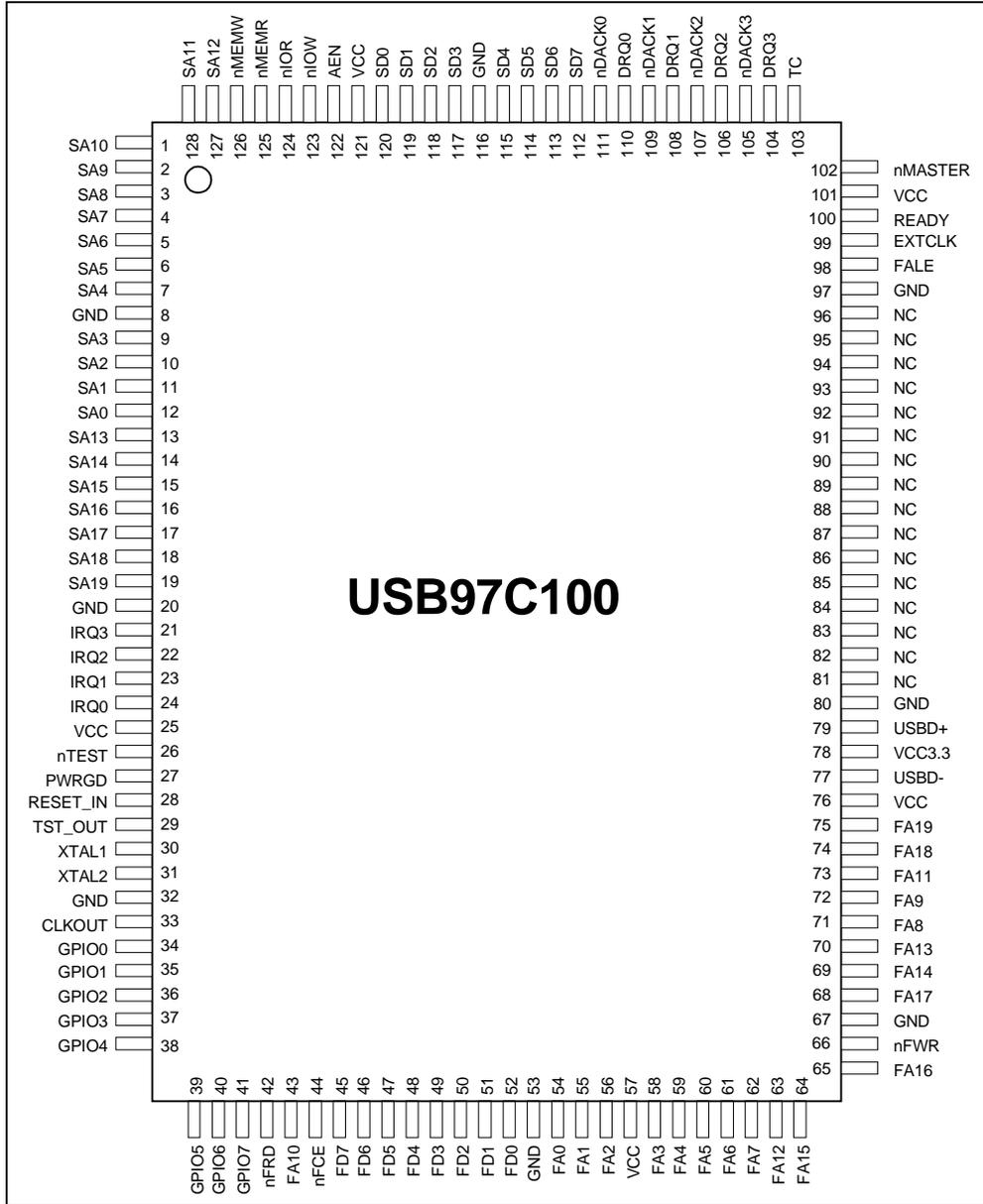
**FIGURE 1 - PIN CONFIGURATION**
