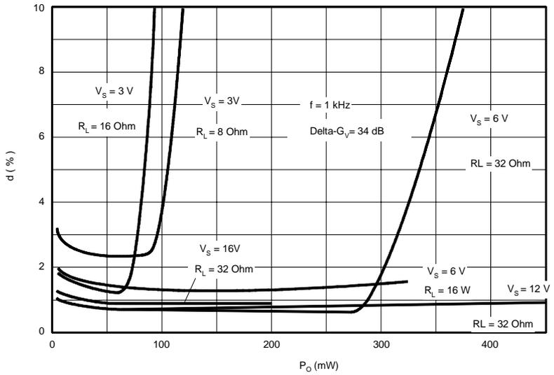
Figure 14. Distortion versus Power —  $f = 3 \text{ kHz}$ ,  $\Delta G_V = 34 \text{ dB}$
