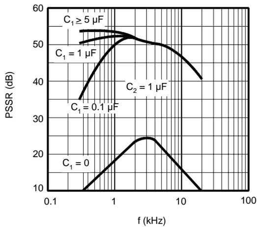
Figure 9. Power Supply Rejection versus Frequency —  $C_2 = 0$
