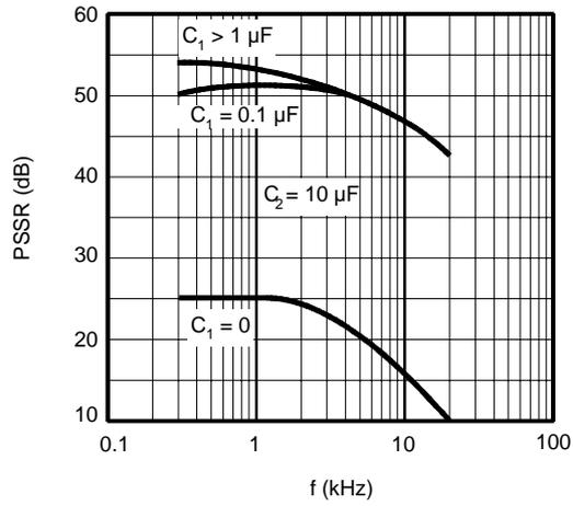
**Figure 7.** Power Supply Rejection versus Frequency —  $C_2 = 5 \mu\text{F}$
