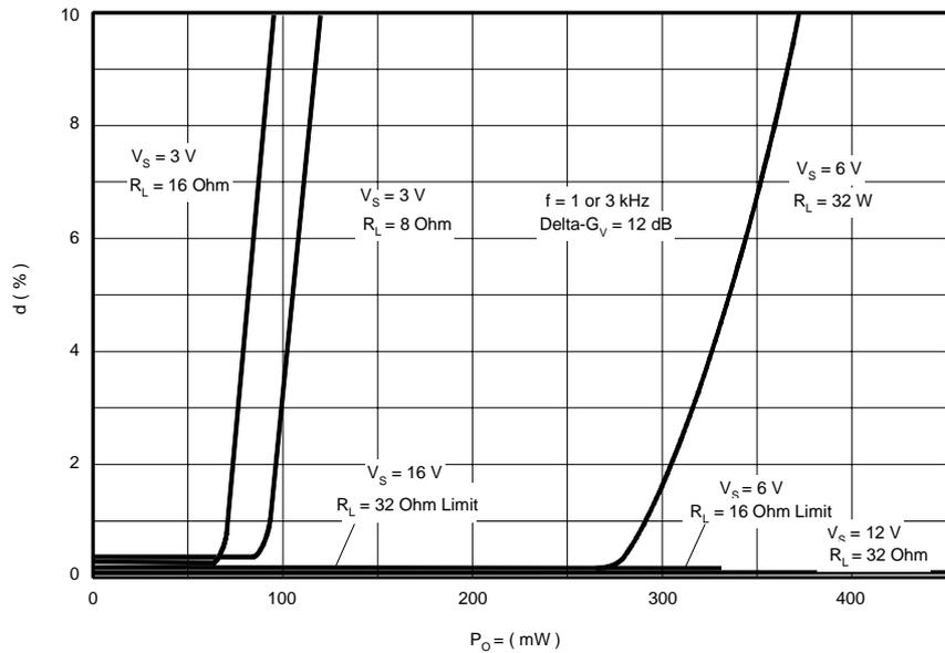
**Figure 16. Maximum Allowable Load Power**
