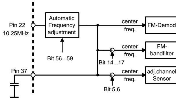
For fine tuning, the center frequency of all these integrated active filters (band filter, demodulator and adjacent channel sensor) can be shifted in steps of 6.25 kHz by means of Bit 56 to Bit 59. Additionally, the center frequency of the band filter can be adjusted separately by means of Bit 14 to Bit 17 if Bit 4 is set to 1. If Bit 4 is set to 0, the default setting is used.
