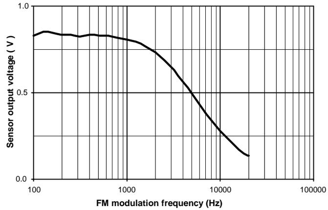
**Figure 17.** FM Input Level Sweep
