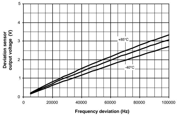
**Figure 16.** Deviation Sensor Frequency Response
