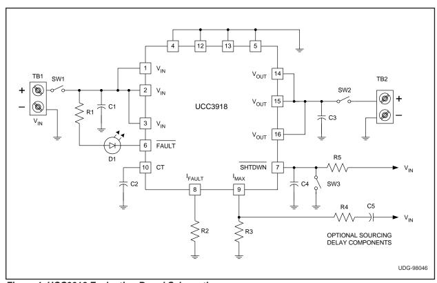
Figure 1. UCC3918 Evaluation Board Schematic
