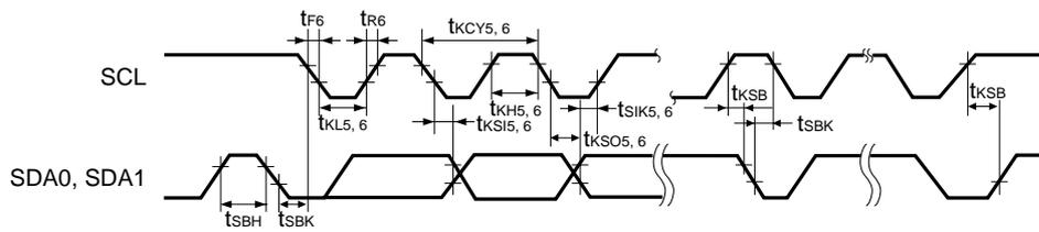
3-wire serial I/O mode with automatic transmission/reception function:
