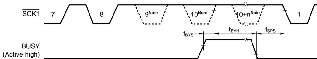
**Note** The signal is not actually low here, but is represented in this way to show the timing.
