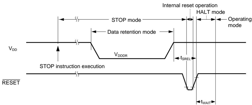
**Data Retention Timing (Standby release signal: STOP mode released by interrupt signal)**
