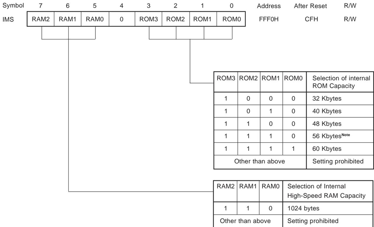
**Note** When the external device expansion function is used, the internal ROM capacity should be set to 56 Kbytes or less.
