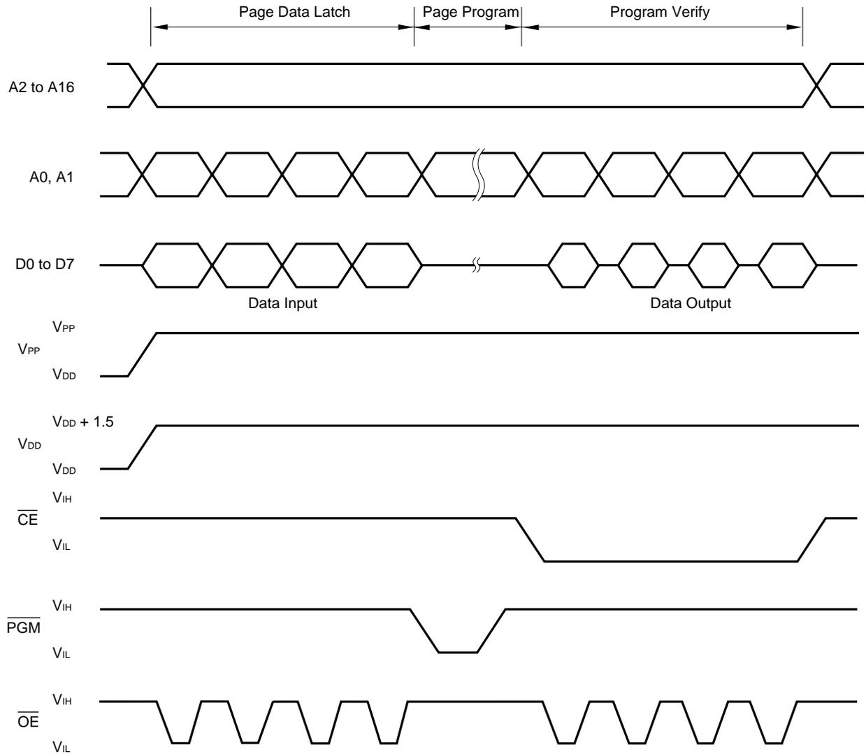
Figure 5-3. Byte Program Mode Flow Chart
