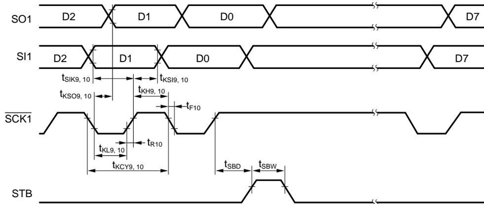
3-wire serial I/O mode with automatic transmission/reception function (busy processing):
