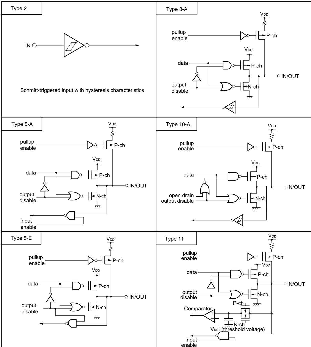
Figure 2-1. List of Pin Input/Output Circuits (2/2)
