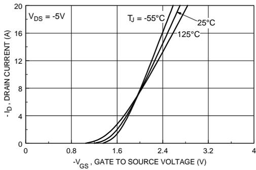
Figure 5. Transfer Characteristics.
