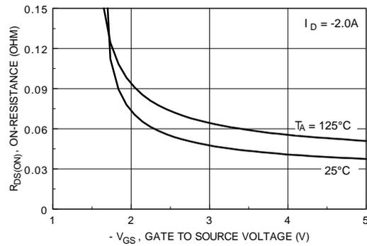
Figure 4. On Resistance Variation with Gate-to-Source Voltage.
