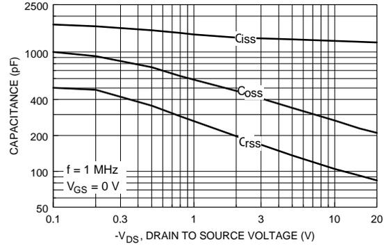
Figure 8. Capacitance Characteristics.
