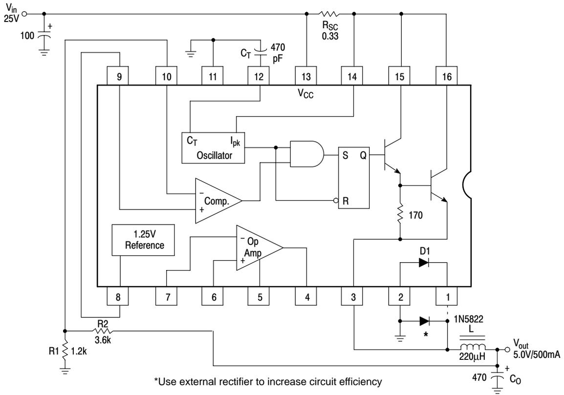
**Figure 6. Step-Down Converter**
