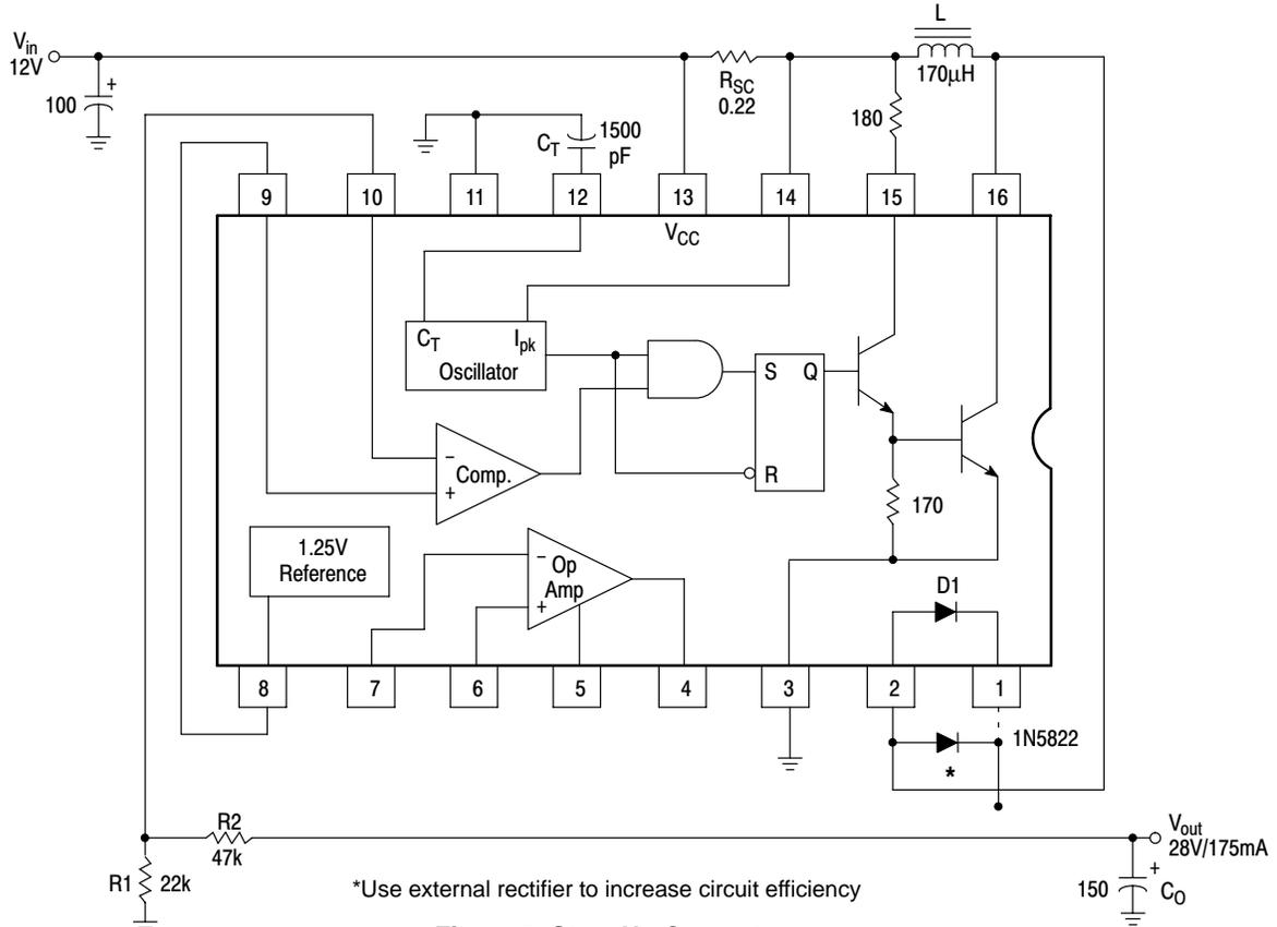
**Figure 7. Step-Up Converter**
