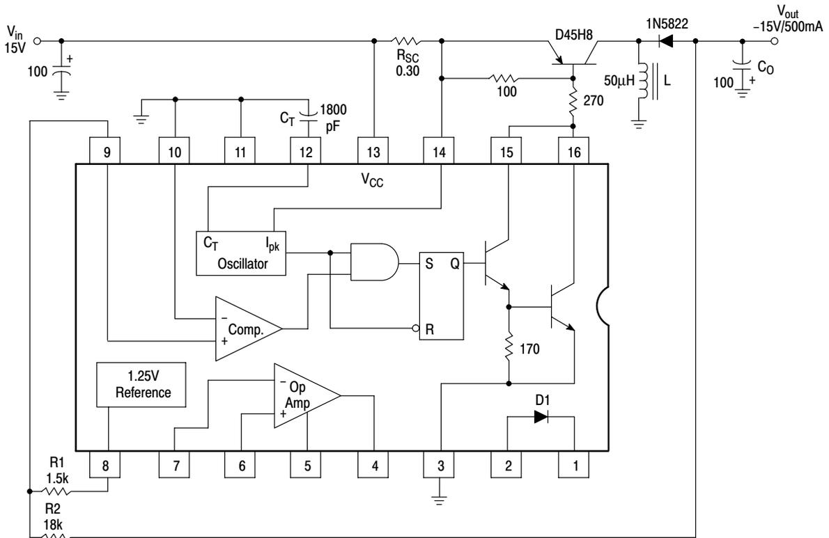
Figure 8. Inverting Converter
