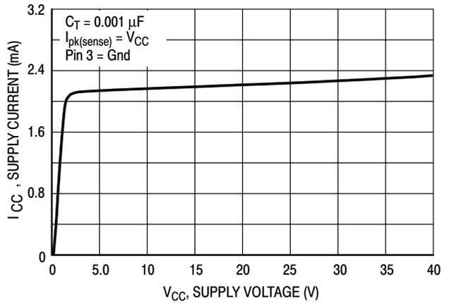
**Figure 3. Standby Supply Current versus Supply Voltage**
