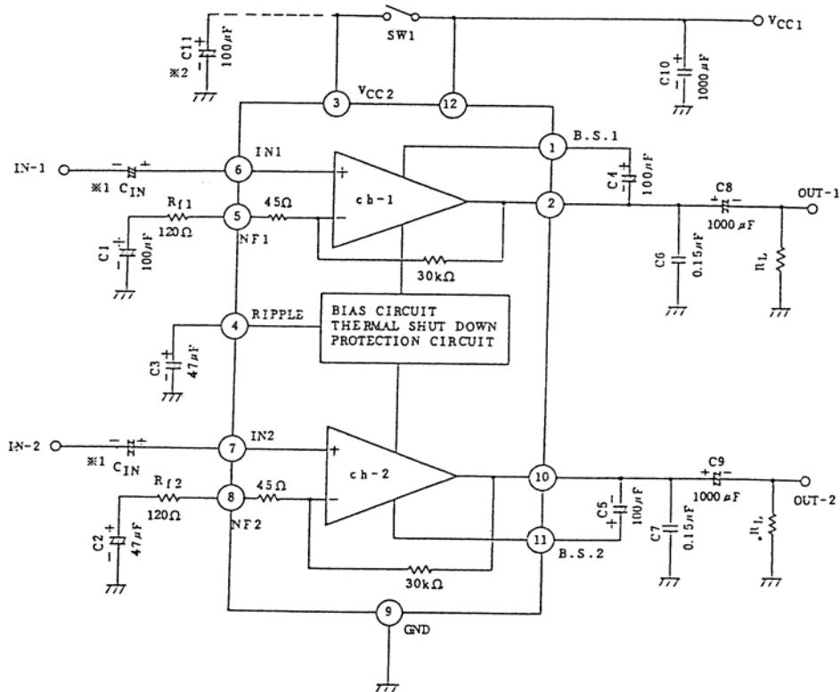
REMARK 1 : This IC can be used without coupling capacitor (CIN). If volume slide noise occurred by input offset voltage is undesirable, it needs to use the capacitor (CIN).
