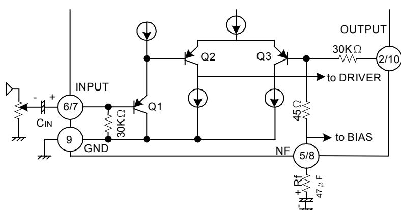
PNP Tr:Q1 is provided in the input circuit so as to make its usage possible without the input coupling capacitor. However, at pin(6) and (7), max 60mV offset voltage is produced.
