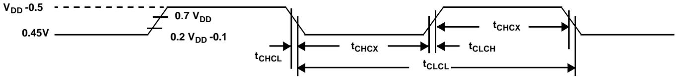
**Figure 5. Clock Signal Waveform for  $I_{DD}$  Tests in Active and Idle Modes**
