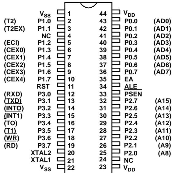
Figure 2b. UT69RH051 44-Pin Flatpack Connections
