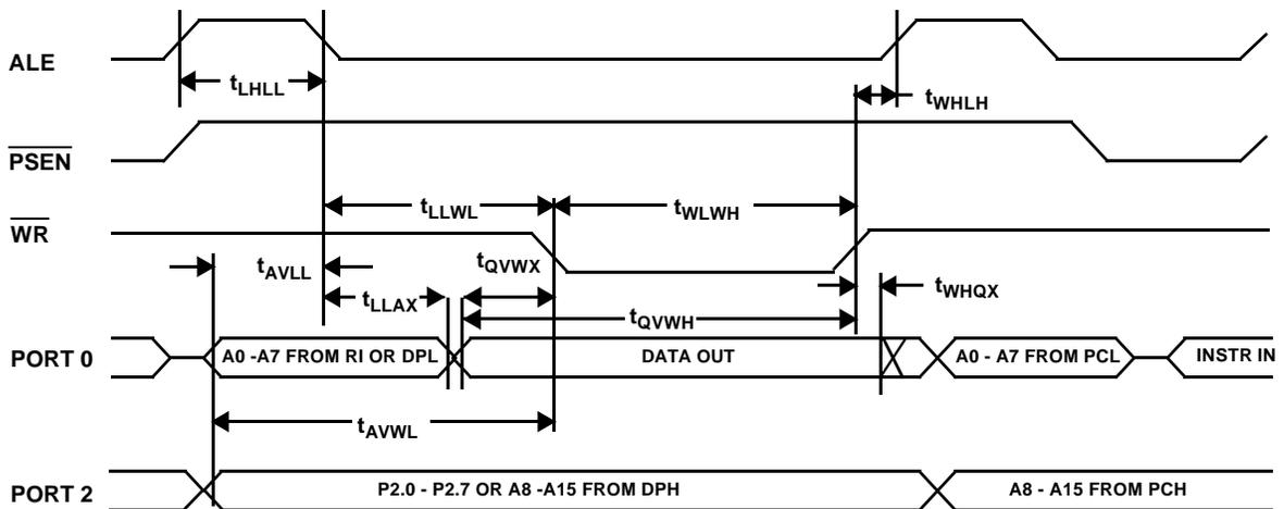
Figure 8. External Data Memory Write Cycle Waveforms
