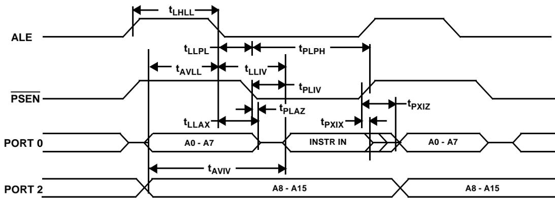
Figure 6. External Program Memory Read Timing Waveforms
