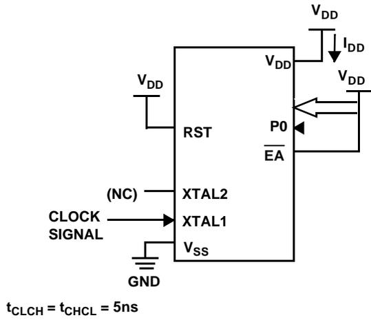
**Figure 4.  $I_{DD}$  Test Condition, Active Mode**
