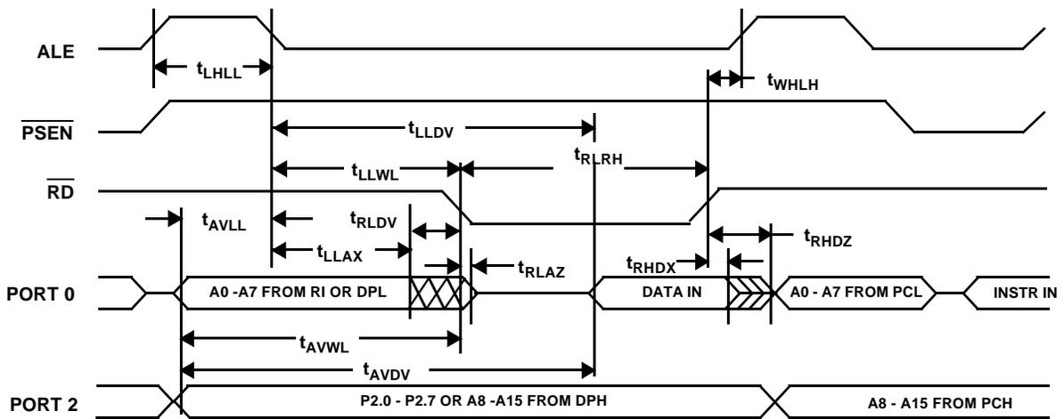
Figure 7. External Data Memory Read Cycle Waveforms
