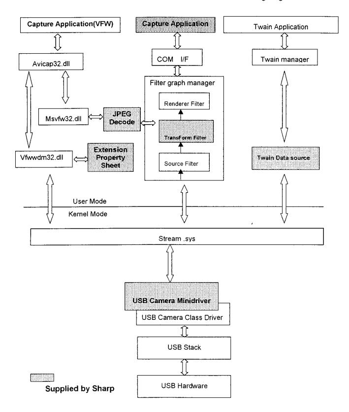
Data and Control Signal Flow is shown below.
