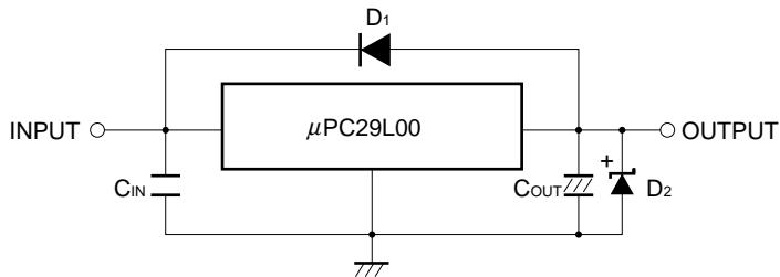
$C_{IN}$  : 0.1 to  $0.47\text{ }\mu\text{F}$ . $C_{OUT}$  : More than  $10\text{ }\mu\text{F}$ .D<sub>1</sub> : Need for  $V_O > V_{IN}$ .D<sub>2</sub> : Need for  $V_O < GND$ .
