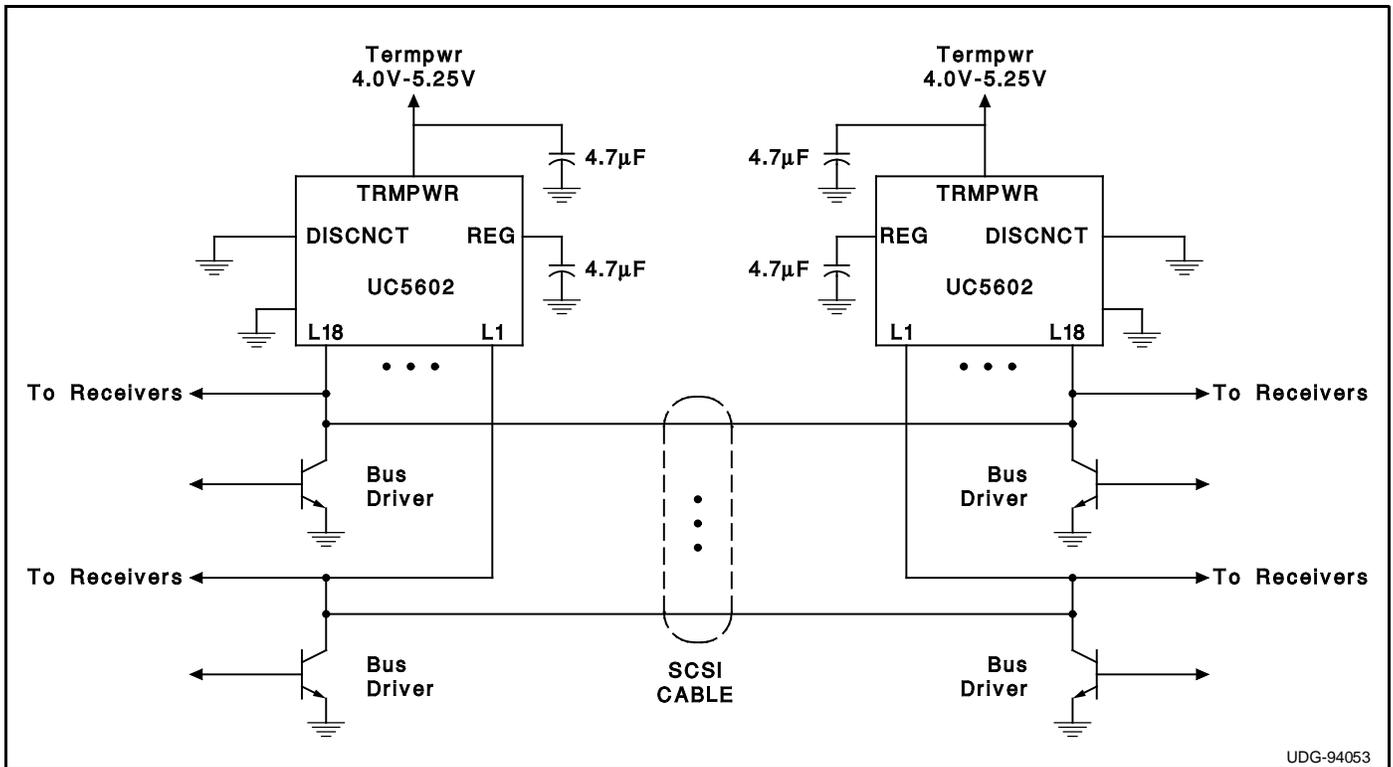
Typical SCSI Bus Configuration Using the UC5602
