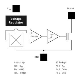
Note: Static sensitive device, please observe ESD precautions. Reverse  $V_{DD}$  protection is not included. For reverse voltage protection, a  $100\Omega$  resistor in series with  $V_{DD}$  is recommended.
