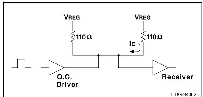
Figure 1. A Single Line of a SCSI Cable
