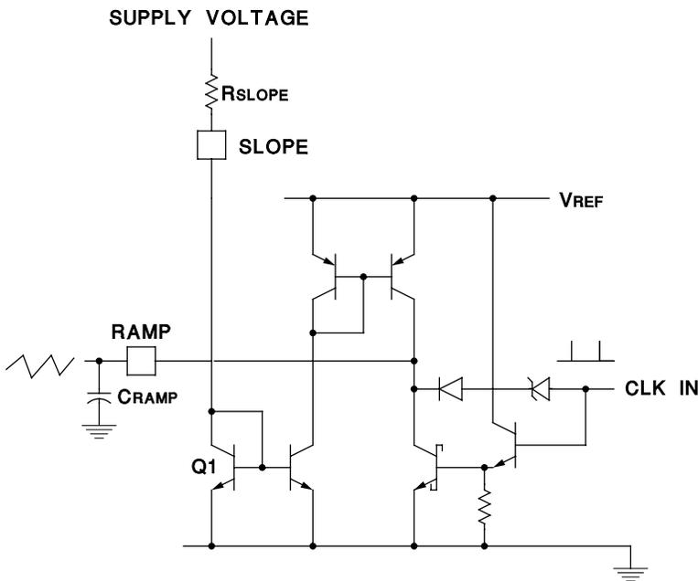
1. Simple voltage mode operation achieved by placing  $R_{SLOPE}$  between  $V_{IN}$  and  $SLOPE$ .
