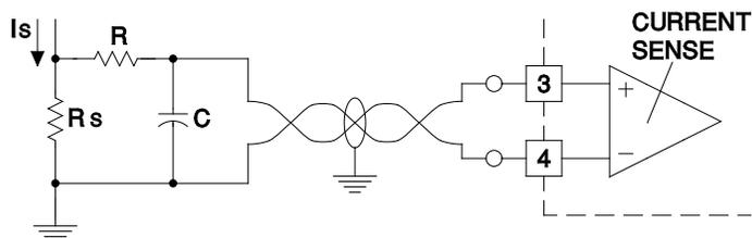
A small RC filter may be required in some applications to reduce switch transients. Differential input allows remote, noise sensing.
