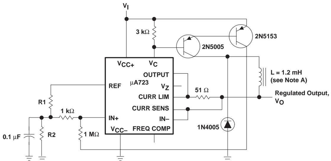
NOTE A: L is 40 turns of No. 20 enameled copper wire wound on Ferroxcube P36/22-3B7 potted core, or equivalent, with a 0.009-inch air gap.
