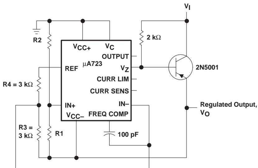
**Figure 3. Negative-Voltage Regulator**
