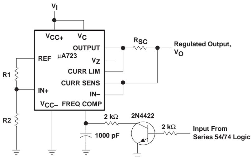
NOTE A: A current-limiting transistor can be used for shutdown if current limiting is not required.
