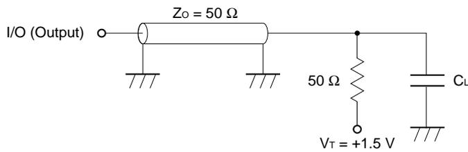
**Remark** CL includes capacitances of the probe and jig, and stray capacitances.
