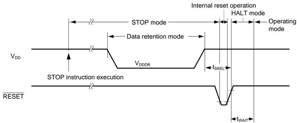
**Data Retention Timing (Standby release signal: STOP mode released by interrupt signal)**
