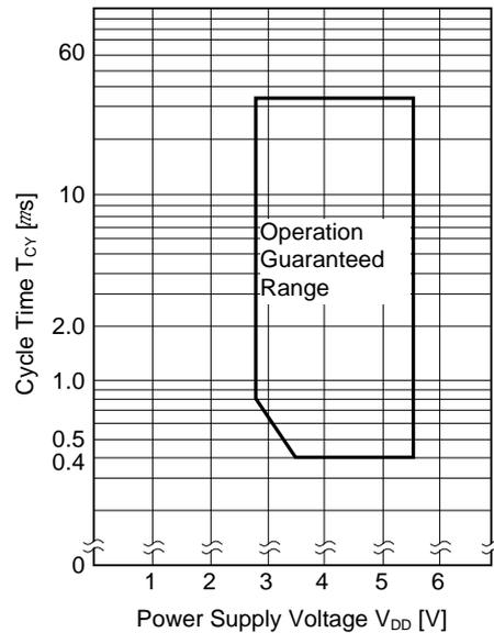
(2) Serial Interface (T<sub>A</sub> = -40 to +85°C, V<sub>DD</sub> = 1.8 to 5.5 V)
