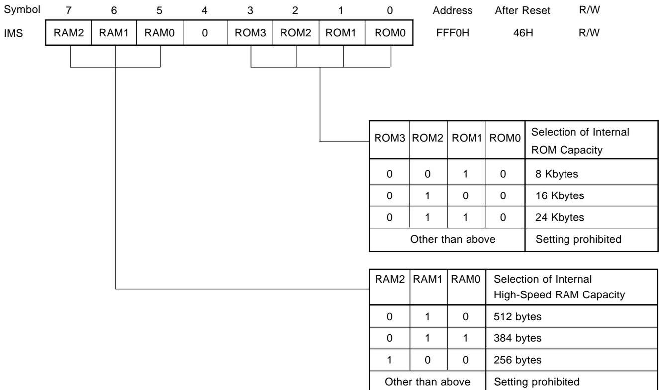
Table 3-1 shows the setting values of IMS which make the memory mapping the same as that of the mask ROM version.
