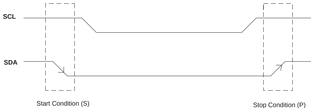
Figure 1. I 2 C Start and Stop Condition
